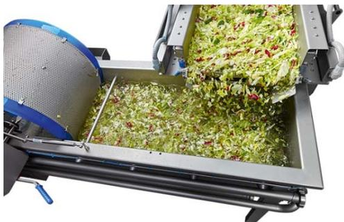
Increasing consumers' safety by hygienizing the process water used during the washing cycle of Fresh-cut salads – without additives, this is the goal of the SiMoHyP project
