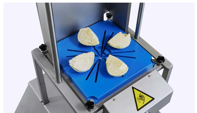
punched into the appropriate shape. The cut product falls down into a prepared container or onto a conveyor belt.
