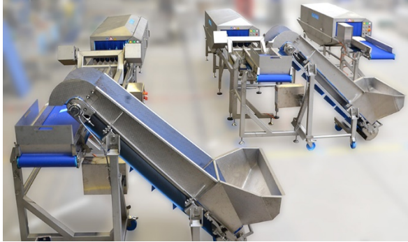
The three UVC Lock lines ensure optimum hygiene before reaching the next processing steps.
