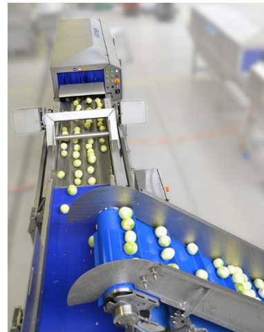
The peeled onions are separately passed through the conveyor belts and vibrating table before being fed into the UVC Lock.
