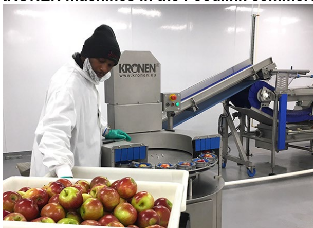
The apple processing line at Foodlink includes a TONA S180K with outfeed belt which connects it to the KDB 120 dipping bath.
