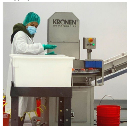
One employee is needed to operate the TONA S180K, placing the apples in the product holders.
