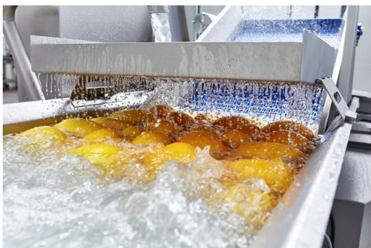
The machines and processing lines produced by KRONEN GmbH and its partners are used to process lettuce, fruit and vegetables: from preparation, cutting, washing, drying, dewatering, peeling and disinfection right through to packaging. Here, for example, whole melons are being washed and disinfected.
