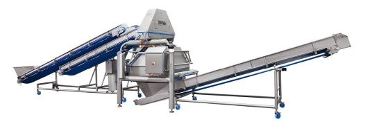
In addition to the new products, a multitude of classic systems and well-established machines will also be demonstrated at the event, including the GS 10-2 (pictured) and GS 20 belt cutting machines. These multifunctional machines can cut an extremely wide variety of foods – including, of course, lettuce, fruit and vegetables – effectively, precisely and gently and with a capacity of up to 1,500 kg/h (GS 10-2) or 4,000 kg/h (GS 20).
