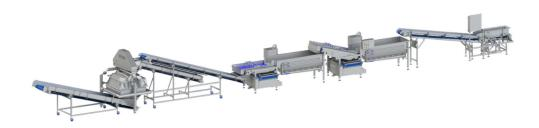
A high capacity of up to 8,000 kg per hour: the KUJ HC-220 cube, strip & slice cutting machine cuts large quantities of fruit, vegetables, and other foods. The machine also processes large products with a diameter of up to 220 mm with the highest cutting quality.
