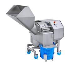
The HEWA 3800 HELICAL washing machine for lettuce, fruit, vegetables, herbs and other foods has been optimized in terms of hygiene and easy cleaning. The design concept also ensures maximum hygiene, for example the fact that the machine has no horizontal surfaces whatsoever, thus allowing the water to optimally discharge. What's more, all edges are designed to avoid the formation of biofilm.
