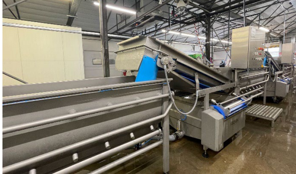
The washing line is comprised of a trimming table and three GEWA 4000 B PLUS HELICAL washing machines and was fitted into the existing production hall.
