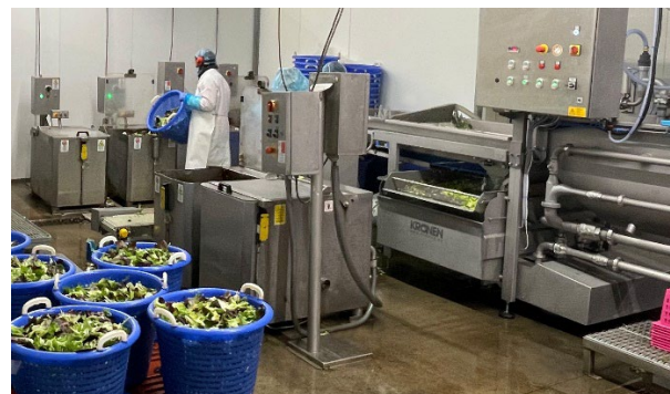
In the washing line, the lettuce, which is often heavily soiled, is reliably and gently freed from soil and processed into ready-to-eat products.
