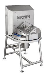
The Tona V is a new cutting solution. It is used to produce slices, segments or sticks from fruit and vegetables. Thanks to several easy-to-change cutting inserts and simple cleaning, it is suitable for frequent cut and pproduct changes. Products to be processed can have a maximum diameter of 120 mm and a maximum height of 150 mm.
