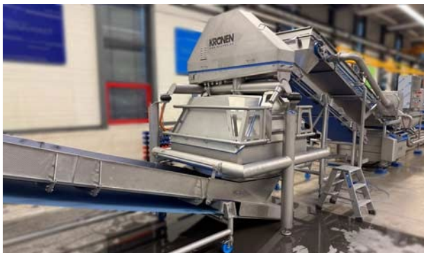
The iceberg lettuce processing line includes a customized K850 drying system from KRONEN.
