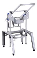
The HGW manual grid cutter can be equipped with various tools. Tropicaux uses the cutting insert to peel and core pineapples.
