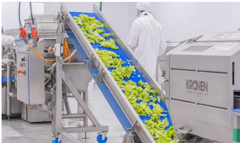
The salad processing line at Comepar includes a GS 10-2 belt cutting machine and a HEWA 3800V PLUS washing machine as well as two KS-100 PLUS spin-dryers.
