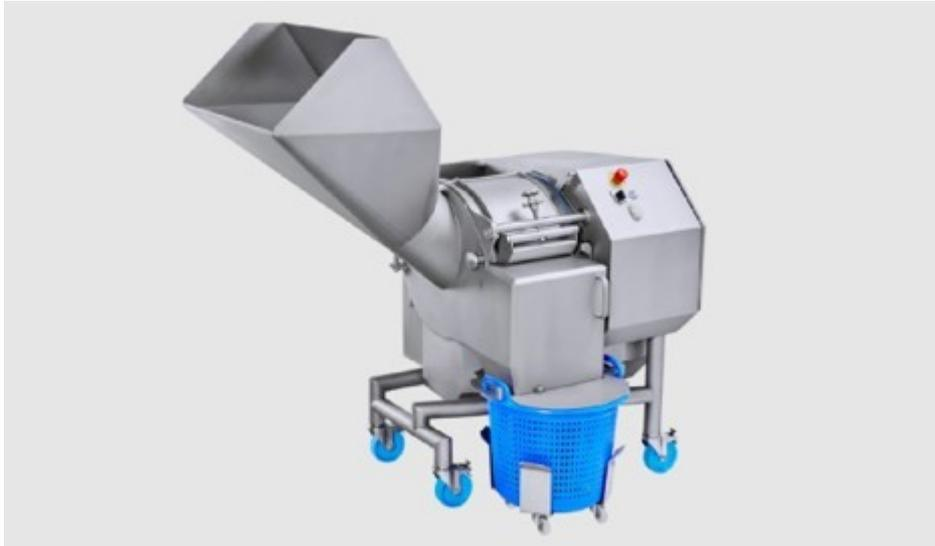
*The new equipment includes the KUJ HC dicer. "Our evaluated dicing machine KUJ has been limited to a cutting width of 85 mm. However, demand is tending more and more towards larger cutting dimensions. Therefore, we have developed the KUJ HC, which was presented for the first time at this year's Fruit Logistica. It has a cutting width of 220 mm, which makes it possible to process whole cabbages, among other things."*
